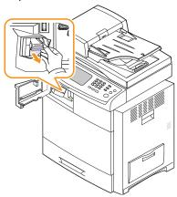
Lift the empty staple cartridge from the stapler unit.
